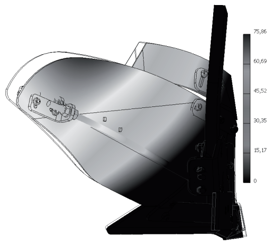
Fig. 18. Rear view of displacement for pressure 0.2 MPa
