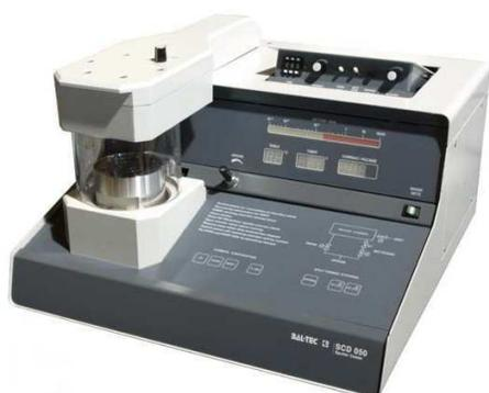
Fig. 3. Sputter coater Bal-Tec company
