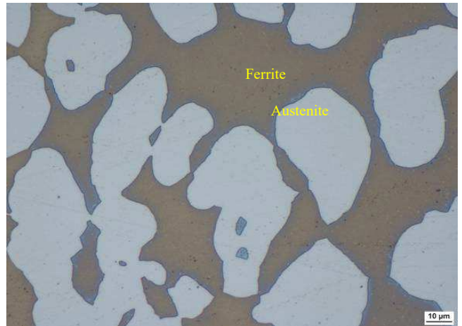
Fig. 4. Specimen A – upon solution-annealing. Etched with NaOH solution
