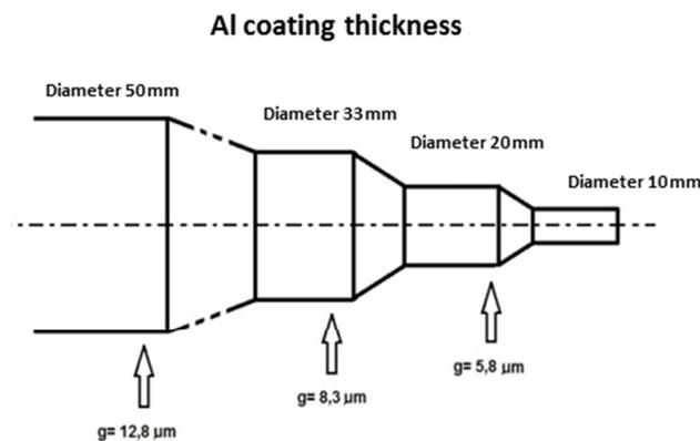
Fig. 4. Diagram of the titanium cylinder after undergoing the hydrostatic extrusion process, titanium with an Al coating having a thickness  $g$ ; first pressing  $\varphi(\text{phi}) - 33 \text{ mm}$ , second pressing  $\varphi(\text{phi}) - 20 \text{ mm}$ , and third  $\varphi(\text{phi}) - 10 \text{ mm}$
