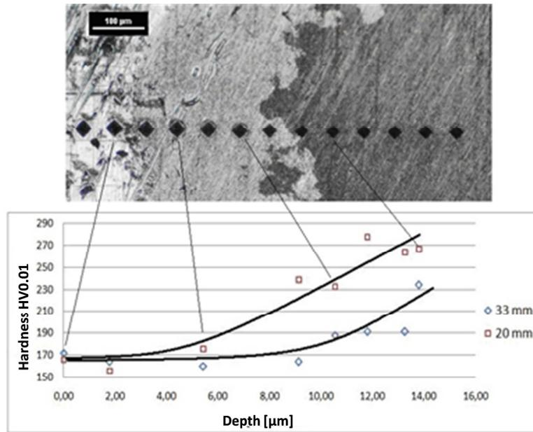
Fig. 8. Profile of the changes in hardness in the surface layer of Grade 3 Titanium covered with an Al coating after the first and second stage of hydrostatic extrusion
