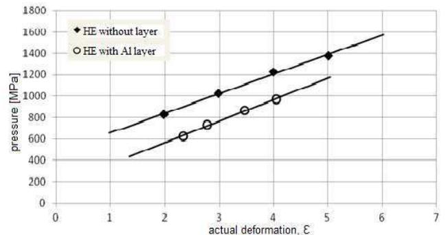
Fig. 2. Pressure dependence as a function of actual deformation for single CP Ti Grade 3 titanium extrusion processes using an Al layer and conventional lubricants
