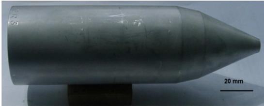
Fig. 3. The original Al coated Grade 3 titanium cylinder with a diameter of 50 mm
