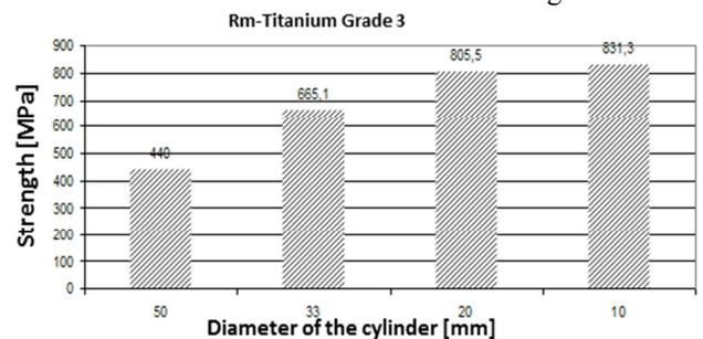
Fig. 10. Tensile strength of hydrostatically extruded Grade 3 titanium
