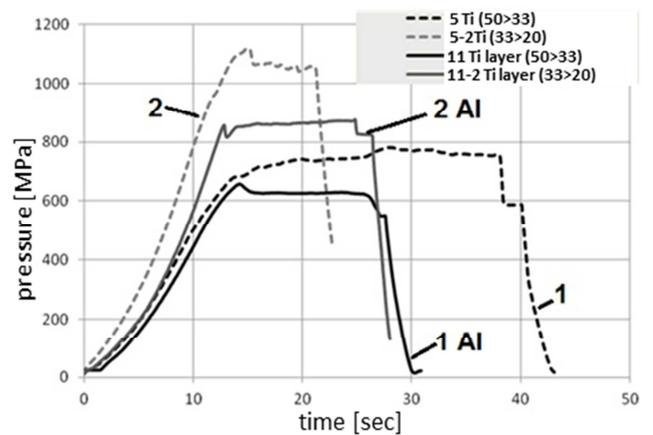
Fig. 1. Pressure characteristics of the hydrostatic CP Ti Grade 3 titanium extrusion process
