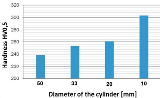
Fig. 9. Core hardness of hydrostatically extruded Grade 3 titanium
