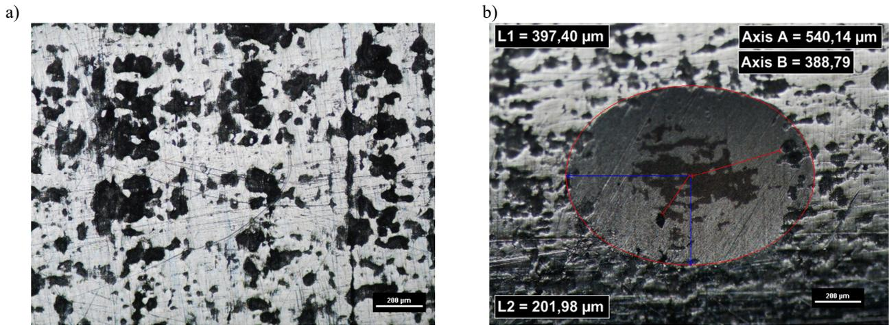
Fig. 5. Cylinder 33 mm, Al coating thickness 8.3 microns, depth 9.7 microns 33 mm
