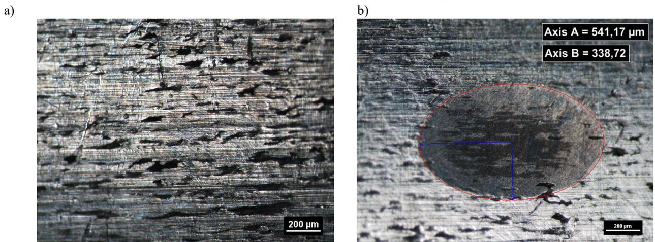
Fig. 6. Cylinder 20 mm, Al coating thickness 5.8, depth of metallographic section 9.7 microns 20 m
