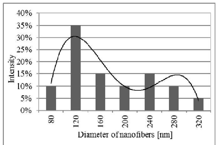
Fig. 8. Nanofibres - Sample 8: a) morphology (SEM), b) measurements of the diameter
