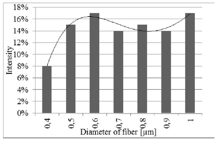
Fig. 5. Microfibrils - Sample 5: a) morphology of the fibers (SEM), b) results of the diameter measurements
