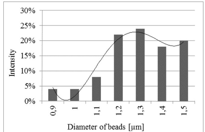
Fig. 1. Fibers with beads- Sample 1: a) morphology of the fiber (SEM), b) results of the diameter measurements
