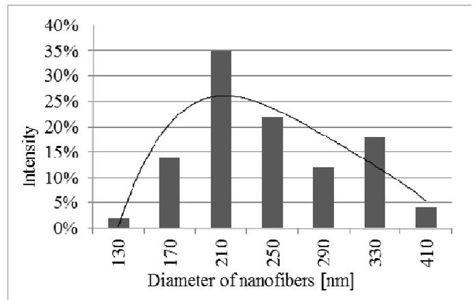
Fig. 7. Nanofibres - Sample 7: a) morphology (SEM), b) measurements of the diameter
