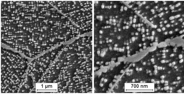
Fig. 5. SEM micrographs of  $M_{23}C_6$  carbides along twins in IN740H after aging at 750°C/1000 h
