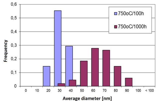
Fig. 7. Size distribution of  $\gamma'$  phase in IN740H after aging at 750°C in different times
