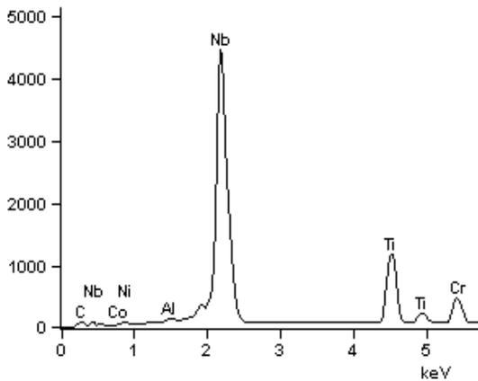
Fig. 2. Chemical composition of MC carbides in IN740H after ageing at 750°C/100 h
