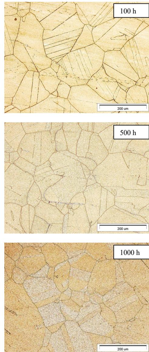
Fig. 1. LM micrographs of samples of IN740H after ageing at 750°C in different times
