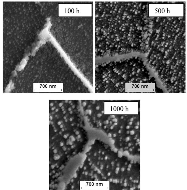
Fig. 4. SEM micrographs of  $M_{23}C_6$  carbides in IN740H after ageing at 750°C in different times
