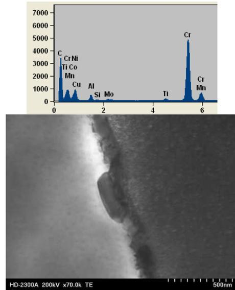
Fig.3. STEM micrograph of  $M_{23}C_6$  carbides in IN740H after aging at 750°C /100 h
