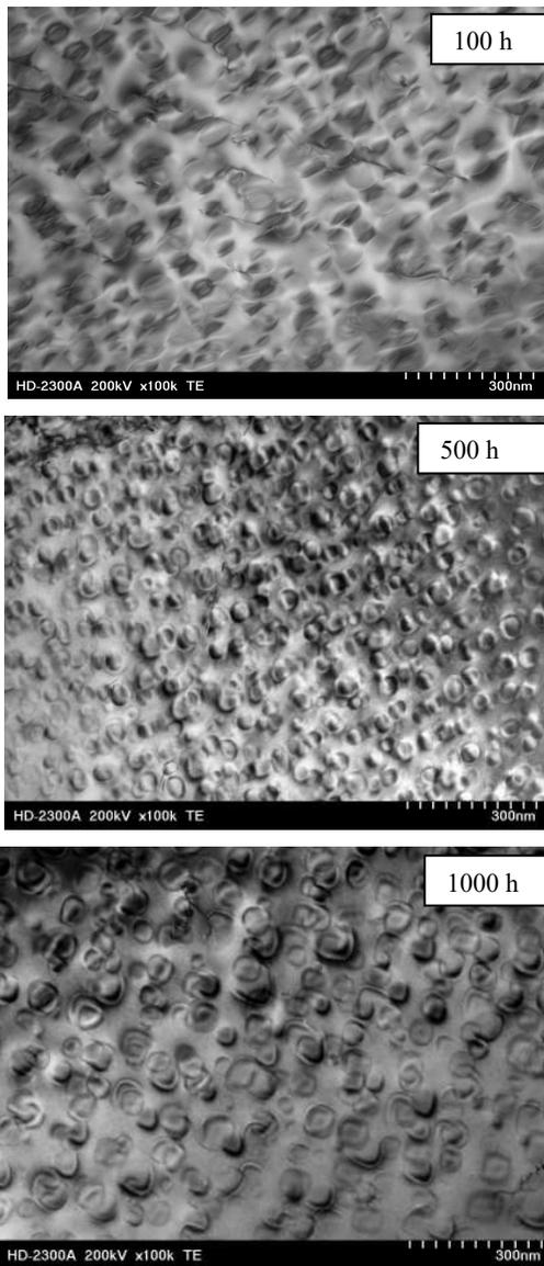
Fig. 6. STEM micrographs of  $\gamma'$  phase in IN740H after aging at 750°C in different times
