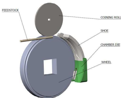
Fig. 1. Description of the 3D model of Conform process
