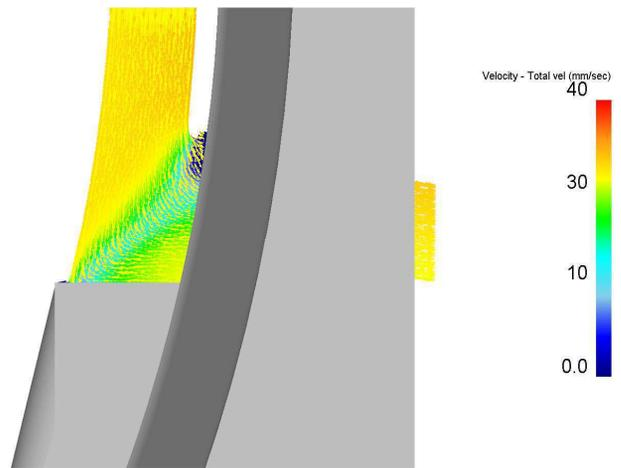
Fig. 3. Material flow in the gap between the wheel and the chamber die
