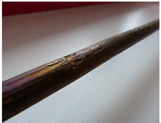
Fig. 5. Damaged surface on the upper side of the extruded wire
