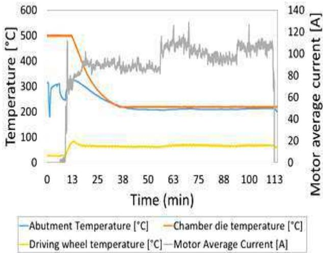
Fig. 2. Temperature curves for the main parts of the Conform machine during extrusion as measured by thermocouples
