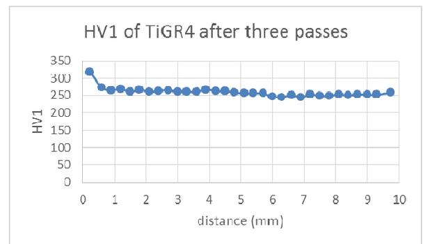
Fig. 8. Micro-hardness profile (after 3 passes)
