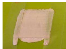
Fig. 4. Titanium dioxide layer prepared by a doctor blade technique
