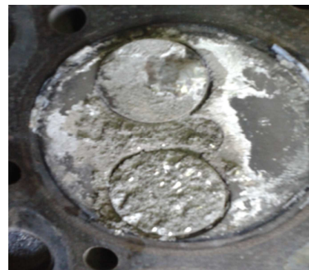
Fig. 4. Gas engine cylinder head after 1500h exploitation without any filter, with deposit caused by siloxanes
