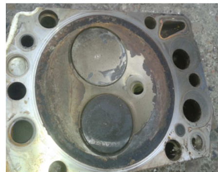
Fig. 5. Biogas engine cylinder head after 1500 h exploitation with micro- and nanostructural multifunctional halloysite-based sorbents from "Dunino" deposit
