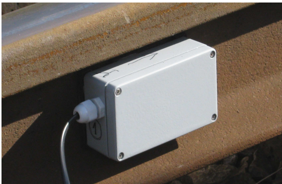
Fig. 2. Accelerometer sensors measuring system
