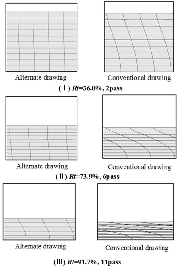
Fig. 8. Transition of element deformation with increasing of  $R_p$  by FEM
