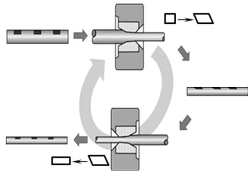
Fig. 1. Alternate wire drawing process
