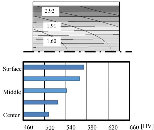
Fig. 10. Relationship of equivalent strain and Vickers hardness by alternate drawing ( $R_t=91.7\%$ )
