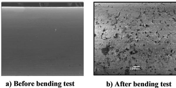
Fig. 14. SEM images of wire surface of conventional drawn wire before and after bending test
