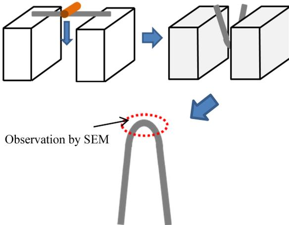
Fig.13 Bending test method
