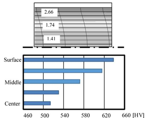
Fig. 9. Relationship of equivalent strain and Vickers hardness by conventional drawing ( $R_t=91.7\%$ )
