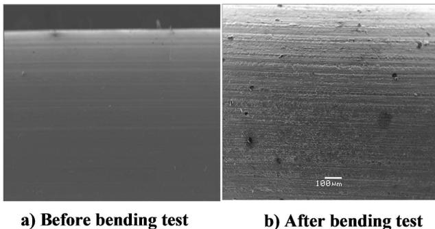
Fig. 15. SEM images of wire surface of alternate drawn wire before and after bending test
