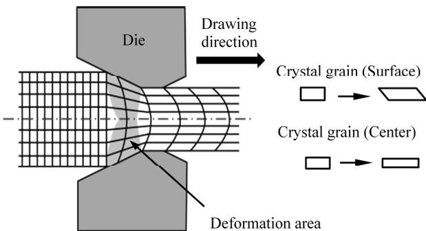
Fig.7. Change of the crystal grain
