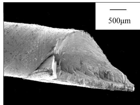
Fig. 11. SEM image of breaking surface of Conventional drawn wire in torsion test
