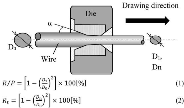
Fig. 3. Definition of wire drawing
