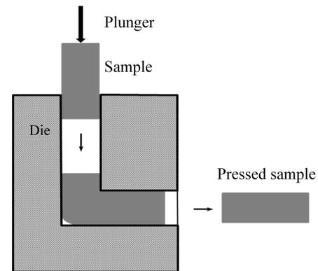
Fig. 2. Equal-channel angular pressing method
