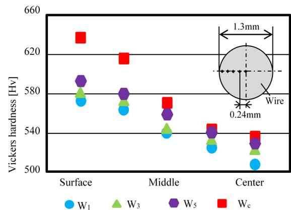
Fig.6 Vickers hardness of several drawn wire (91.7%)
