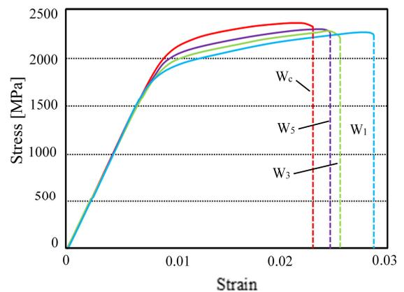
Fig. 5 Stress strain curves of several drawn wire (91.7%)
