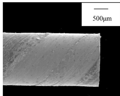
Fig. 12. SEM image of breaking surface of Alternate drawn wire by torsion test
