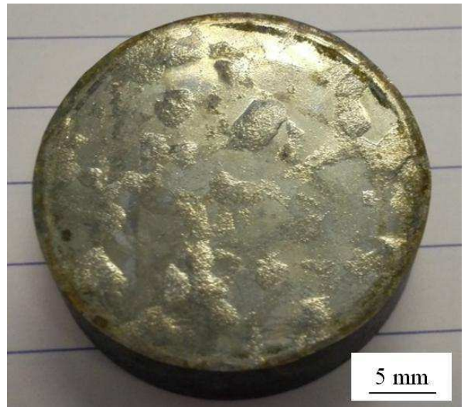
Fig. 5. Macroscopic appearance of Zn-1.6Al-1.6Mg-3Sn after 500h salt spray test
