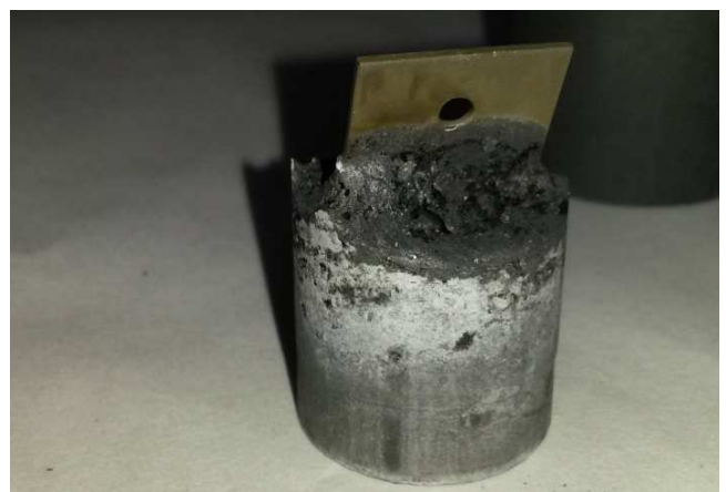
c) MoNiCr specimen no. 6 in solidified salt after the experiment
