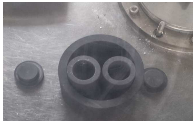
b) Graphite containers in dry box
