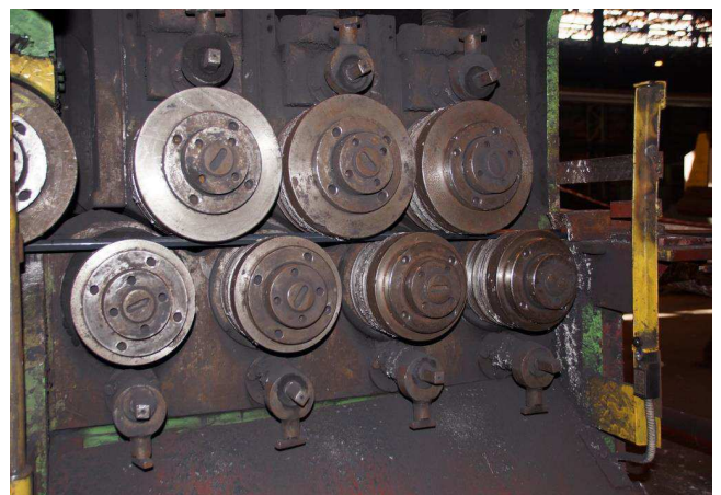
Fig. 1 Roller straightener with a straightened by bending rod. Above and below straightener rods conspicuous mandrels for vertical control of the rolls
