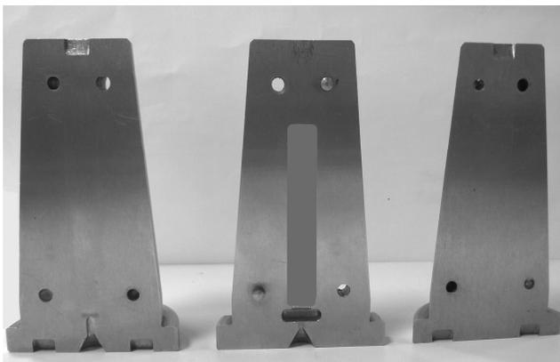
Fig. 3. Injection molded part in three plate mold
