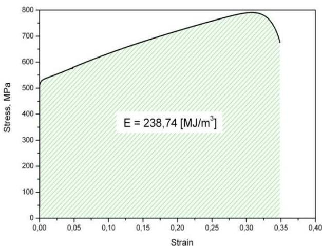
Fig. 4. Representative tensile curve for a steel X8MnSiAlNbTi25-1-3 with designated strain energy per unit volume after the cold plastic deformation
