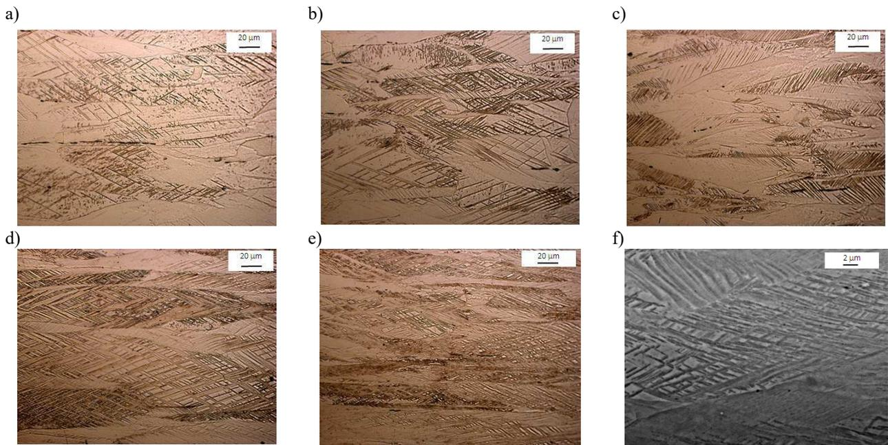
Fig. 1. Structures of the investigated X8MnSiAlNbTi25-1-3 steel after the static tensile test stretched to a predetermined elongation of a) 5%, b) 10%, c) 20%, d) 30%, and e), f) after sample breaking
