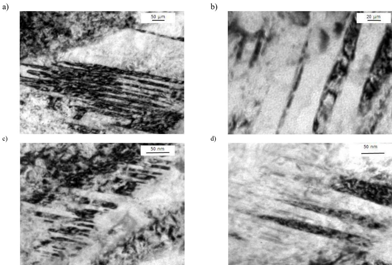
Fig. 2. Twinned austenite area in the structure of thin films in X8MnSiAlNbTi25-1-3 steel after the static tensile test stretched to a predetermined elongation of a-d) 20%
