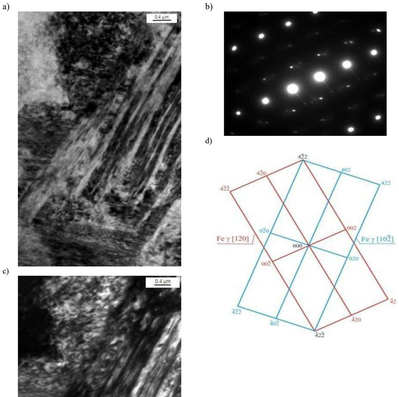
Fig. 3. Deformation twins intersecting in two different systems in the thin foil structure of the X73MnSiAlNbTi25-1-3 steel, steel structure observed in transmission electron microscope after static tensile test until break; a) bright field, b) diffraction pattern from the area in Fig. a), c) the dark field from the spot(002)  $\text{Fe}_\gamma$  from the area presented in Fig. a); d) solution of the diffraction pattern
