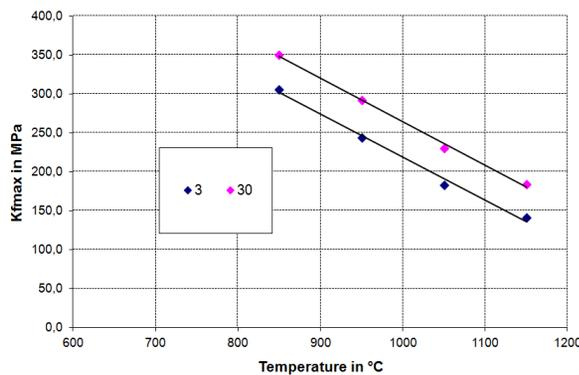
Fig. 10. Results of Rastegaev compression test
