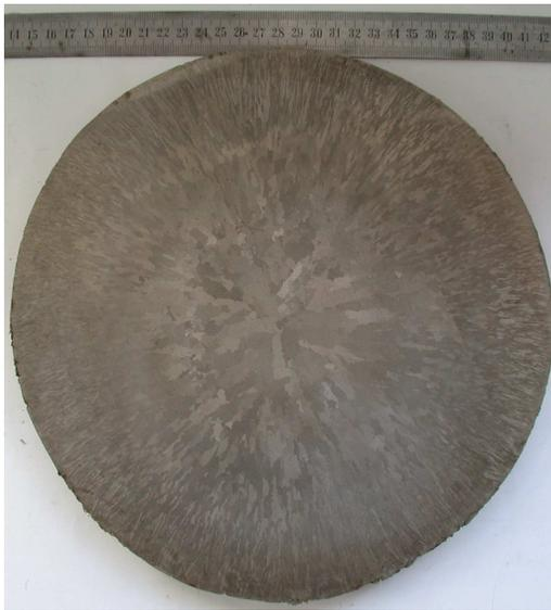
Fig. 1. Macrostructure of ingot
