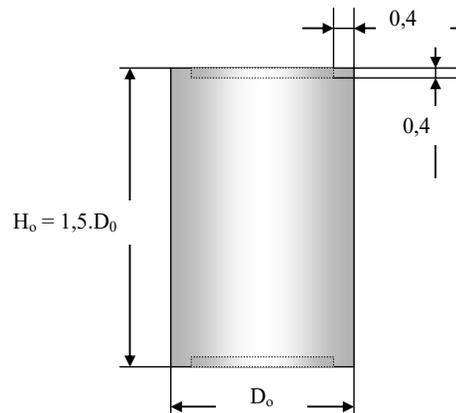
Fig. 7. Rastegaev sample geometry [7]
