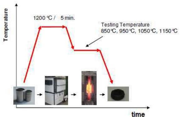
Fig. 8. Process of Rastegaev compression test
