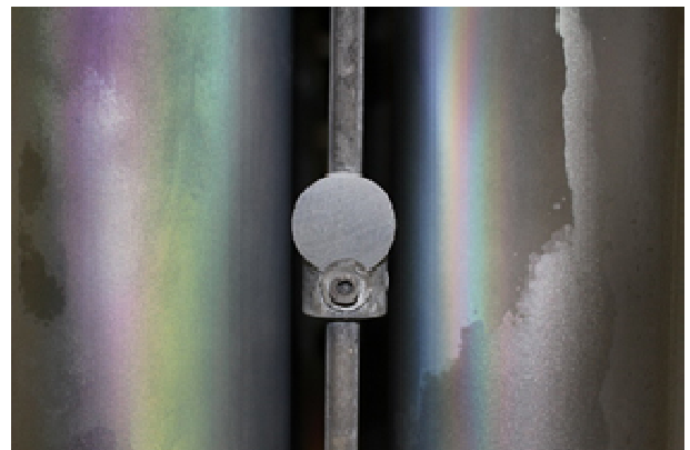
Fig. 2. Specimen holder with PA6 sample
