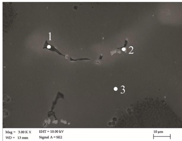
Fig. 2. SEM micrograph of the AlMg3 alloy in initial state and EDS spectra of corresponding points
