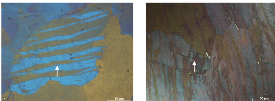
Fig. 6 Microstructures of AlMg<sub>3</sub> alloy after ECAP process showing a) shearing bands, b) slip lines
