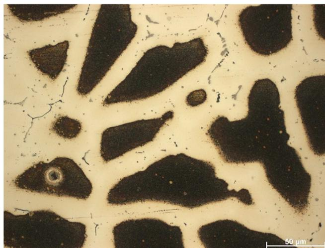
Fig. 1. Structure of AlMg3 in initial state (as cast) a) polarized light (Barker's reagent), b) bright field (Weck's reagent)
