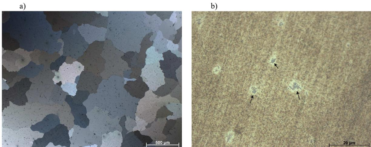
Fig. 3. Structure of the AlMg3 alloy after artificial ageing a) polarized light (Barker's reagent), b) bright field (Weck's reagent)
