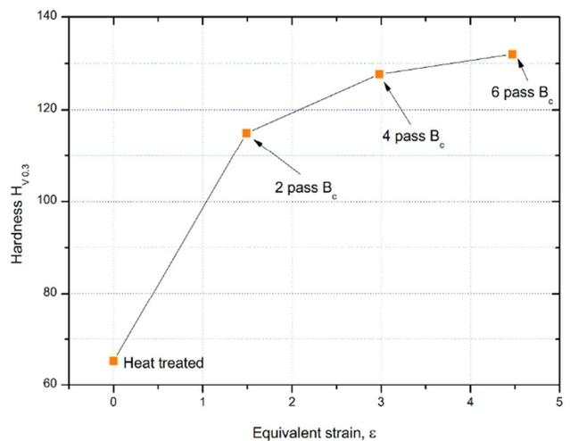
Fig. 8. Variation of the hardness Hv, with the equivalent strain and number of passes
