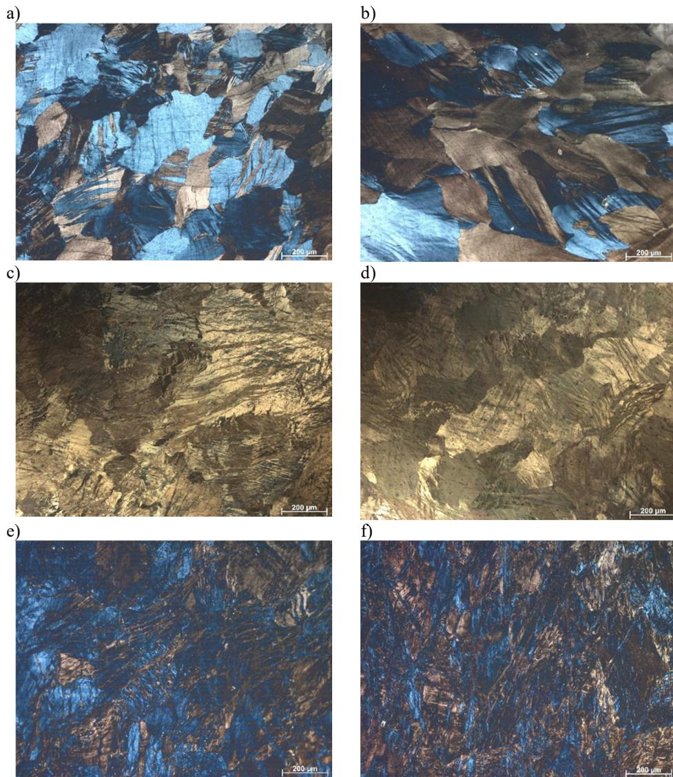
Fig. 5. Structure of the AlMg<sub>3</sub> alloy after heat treatment and ECAP process a) 2 pass (X-plane), b) 2 pass (Y-plane), c) 4 pass (X-plane), d) 4 pass (Y-plane), e) 6 pass (X-plane), f) 6 pass (Y-plane)
