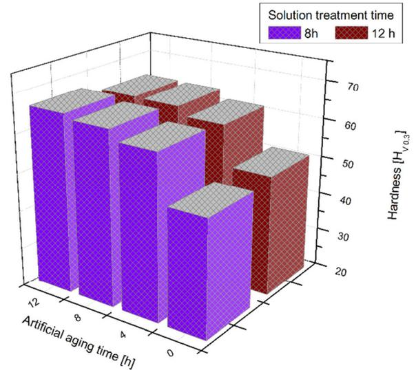
Fig. 7. Effect of heat treatment on the hardness of AlMg3 alloy
