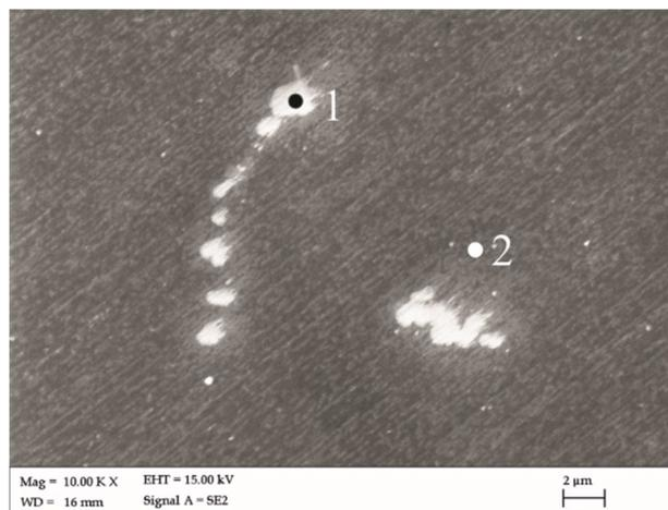
Fig. 4. SEM micrograph of the AlMg3 alloy in initial state and EDS spectra of corresponding points
