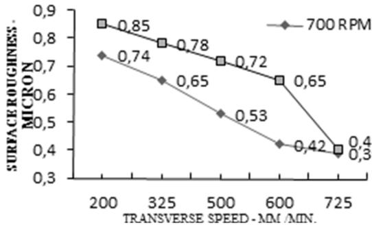
Fig. 7. Transverse vs surface roughness at 700 and 1120 RPM
