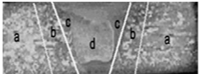
Fig. 2. Different zones of FSW: (a). Base metal, (b).Heat Affected Zone (HAZ), (c).Thermo – Mechanically Affected Zone, and (d). Nugget zone [15-16]
