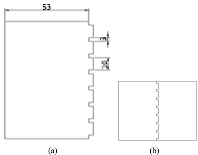
Fig. 3. Square groove specimen (a) and (b) as welded
