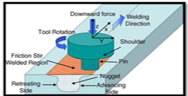
Fig.1. Working principle of FSW [14]
