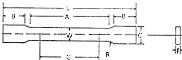
Fig. 6. Test specimen as per ASTM [17]
