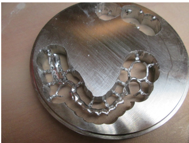
Fig. 8. The denture frame is milled in a metal block
