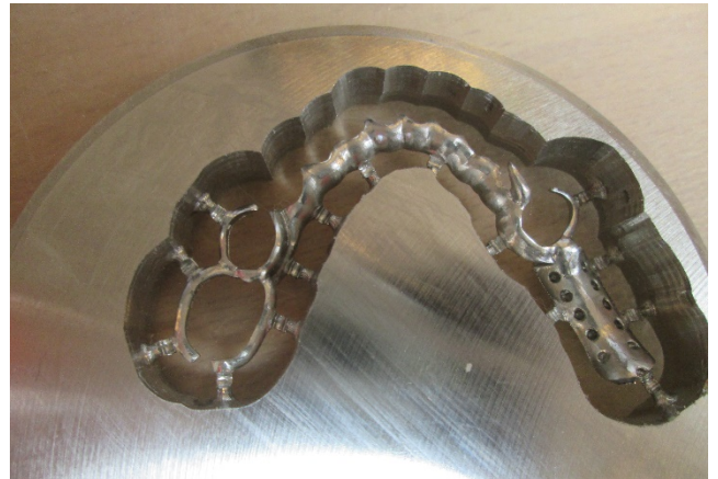
Fig. 9. Connectors linking the denture frame with the metal block must be precisely cut to ensure accuracy of the whole structure
