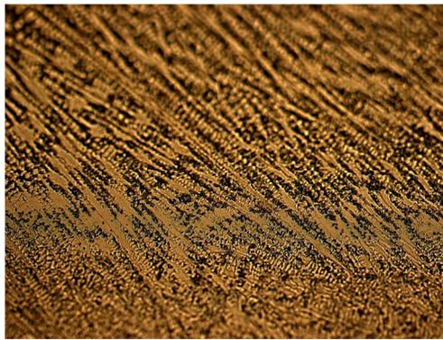
Fig. 7. The structure of the alloy Heraenium NA, magnification 500x
