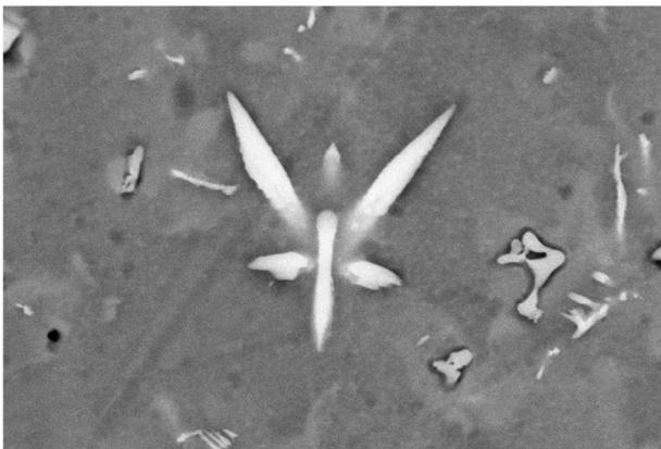
Fig. 3. The structure of the alloy ARGELLOY N.P.BE-FREE - SEM accelerating voltage 20 kV, magnification 2000x
