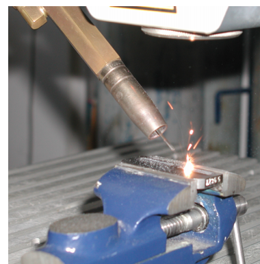
Fig. 1. HPDL laser Rofin DI 020 used for remelting and alloying of the hot work tool steel samples
