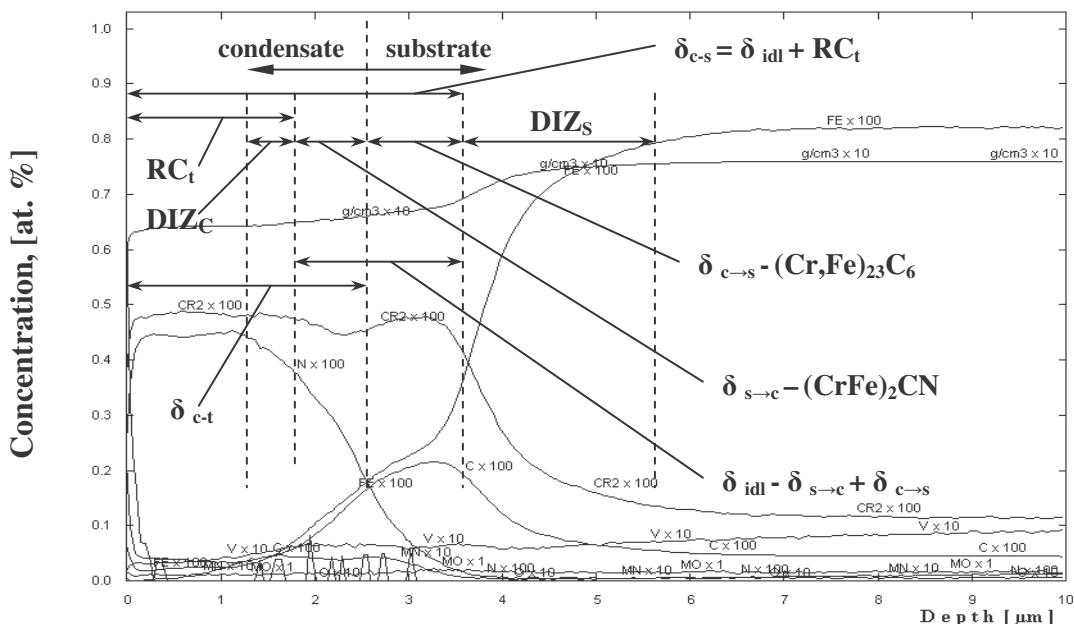
Fig. 2. GDOES profile of CrN coating on X12M steel, obtained at  $T_m = 850^\circ\text{C}$ ,  $L_{t-s} = 70$  mm and  $U_s = 0$  V after heat-treatment.
