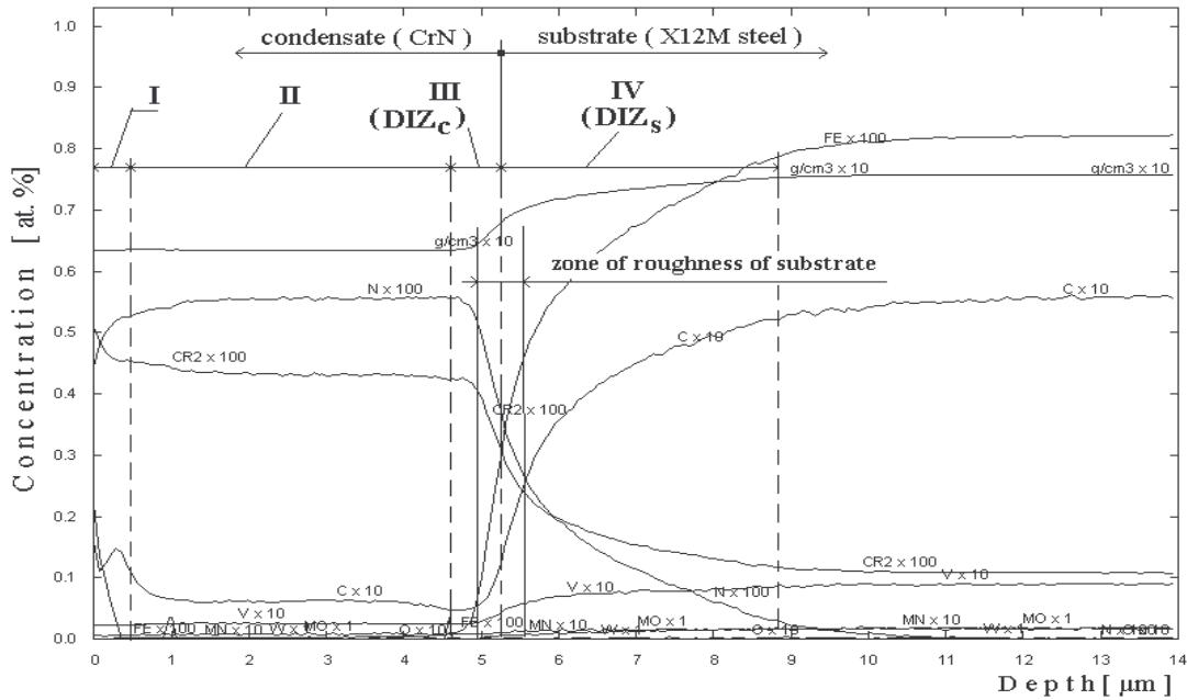
Fig. 1. GDOES profile of a CrN coating on a X12M steel, obtained at T<sub>m</sub> = 450°C, L<sub>t-s</sub> = 70 mm and U<sub>s</sub> = 0 V.
