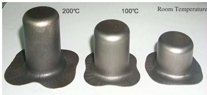
Fig. 10. Drawn cups at various forming temperatures
