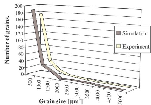
Figure 2. Histogram of the grain size for the specimen of Armco iron deformed 20% and then recrystallized and the microstructure obtained from the simulation for decreasing nucleation rate and  $H/J=1.5$ .
