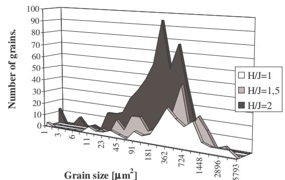
Figure 4. Histogram of the grain size distribution for the calculated microstructures for decreasing nucleation rate and the degree of stored energy  $H/J=1, 1.5$  and  $2$ .
