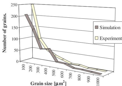
Figure 3. Concentrated histogram of the grain size ranging from 0-1000  $\mu m^2$  for the specimen of Armco iron deformed 30% and then recrystallized and the microstructure obtained from the simulation for decreasing nucleation rate and  $H/J=2$ .
