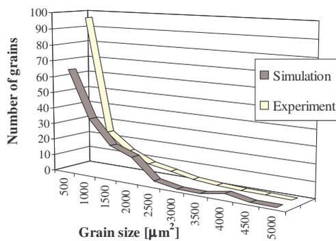
Figure 1. Histogram of the grain size for the specimen of Armco iron deformed 10% and then recrystallized and the microstructure obtained from the simulation for decreasing nucleation rate and  $H/J=1$ .
