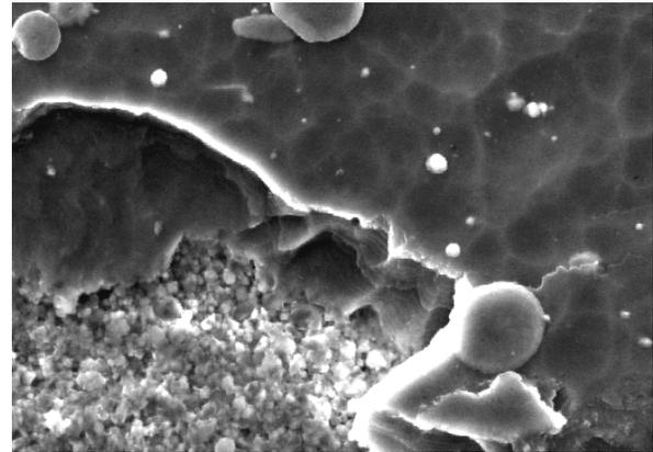
Fig. 6. Characteristic failures of the TiN+multiTiAlSiN+TiN coating deposited onto the T130A type tool cermet
