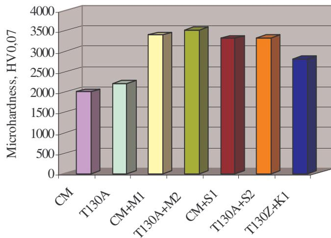
Fig. 3 The HV<sub>0,07</sub> microhardness values for substrate and coating surfaces
