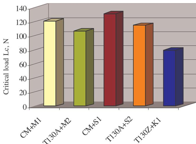
Fig. 4 Critical load  $L_c$  [N] values for the particular coatings (Fig. 5).
