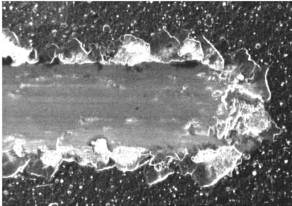
Fig. 5. Indenter trace with the maximum load on the TiN+multiTiAlSiN+TiN coating surface deposited onto the T130A type tool cermet
