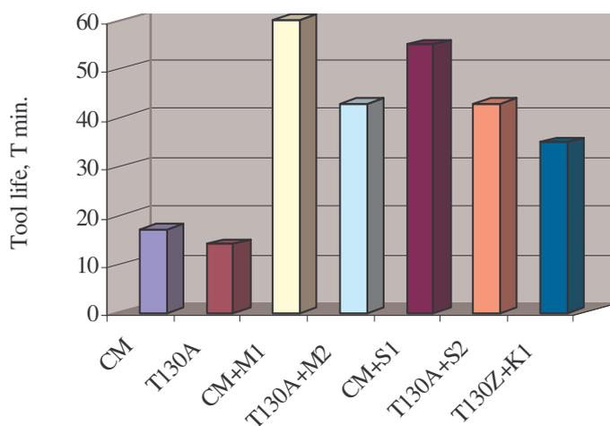
Fig. 7 Tool life T [min] for the particular coatings
