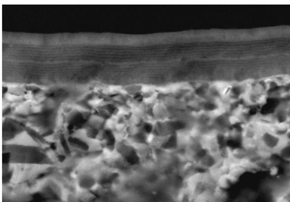
Rys. 1. Fracture surface of the TiN+multiTiAlSiN+TiN coating deposited onto the CM type cermet
