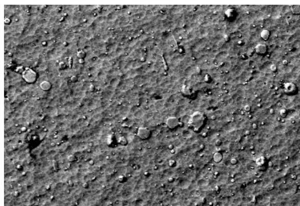
Rys. 2. Surface topography of the TiN+multiTiAlSiN+TiN coating deposited onto the CM type cermet
