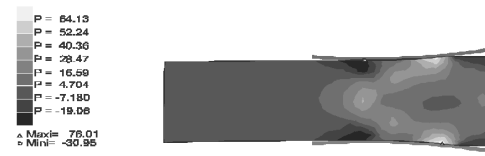
Fig.4. Distribution of stresses \sigma_m within the roll gap, with h_0=105.76 mm, \epsilon=10\% , \theta=2^\circ , positive values means compression
