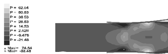
Fig.2. Distribution of stresses \sigma_m within the roll gap, with h_0=105.76\text{ mm} , \epsilon=10\% , \theta=0^\circ , positive values means compression
