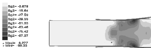
Fig.1. Distribution of stresses \sigma_y within the roll gap, with h_0=105.76\text{ mm} , \epsilon=10\% , \theta=0^\circ
