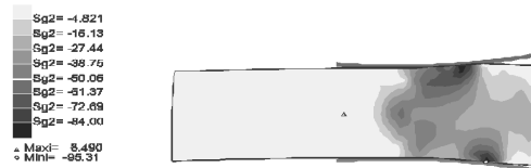
Fig.5. Distribution of stresses \sigma_y within the roll gap, with h_0=105.76 mm, \epsilon=10\% , \theta=4^\circ
