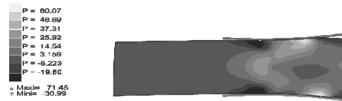
Fig.4. Distribution of stresses \sigma_m within the roll gap, with h_0=105.76 mm, \epsilon=10\% , \theta=2^\circ , positive values means compression
