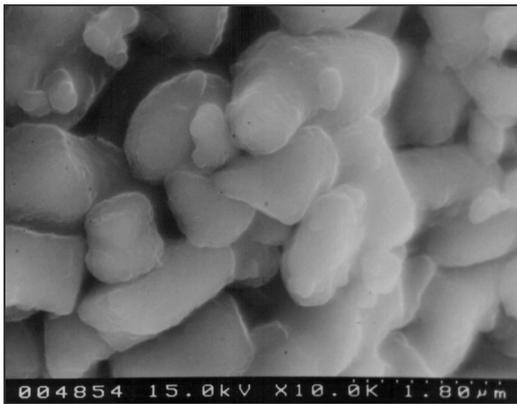
Figure 5. Micro photographs of a single granulate fracture Alcoa CT 1200
