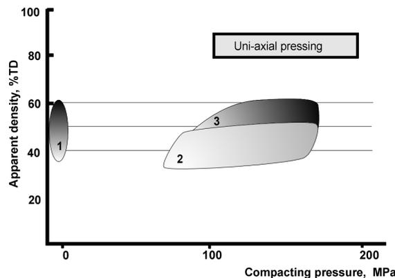
Figure 1 . Specific gravity of ceramic powders die – stampings [1-9].
