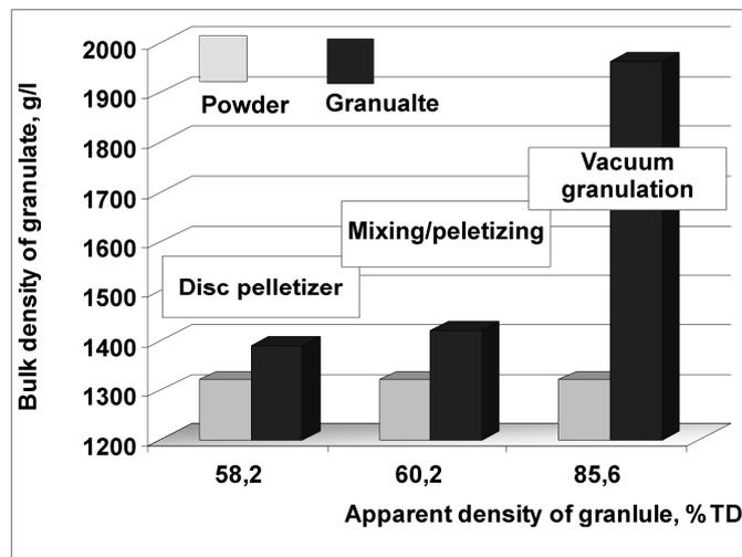
Figure 4 . Comparison of the effectiveness of different granulation techniques
