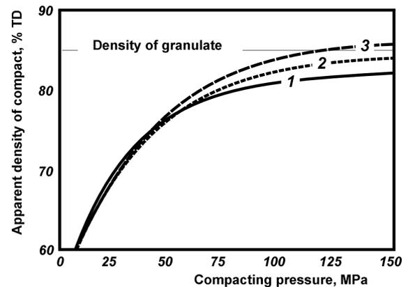
Figure 6. Course of a granulated product concentration process (single axle moulding in matrix) (1), grinded granulated product - below 2 mm (2), grinded granulated product - below 1 mm (3)
