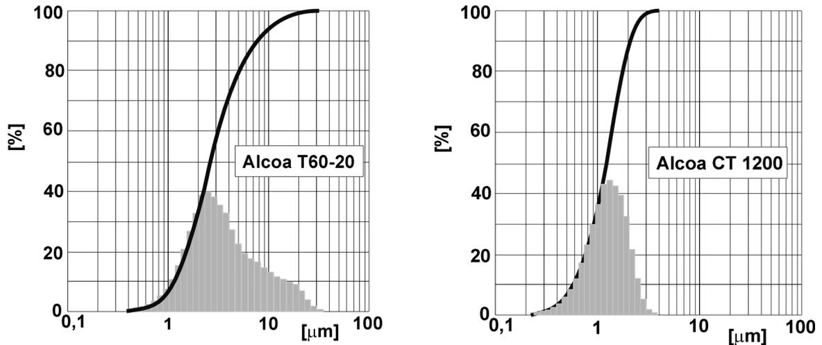
Figure 3. Graining of aluminium oxide powders used in testing effectiveness of vacuum granulation
