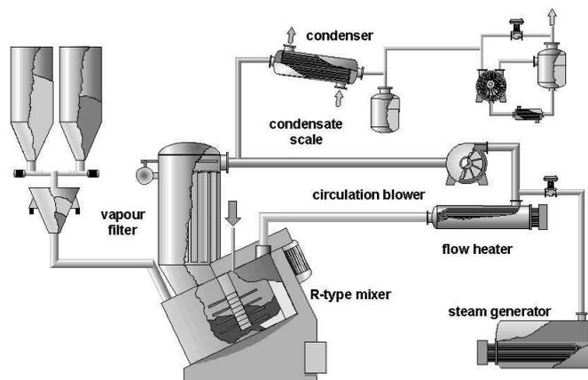
Figure 2 . Diagram of ‘Evactherm’ device [10]
