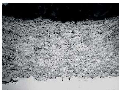
Fig. 1. Light microscopy image of FeAl-Fe x Al y composite coating
