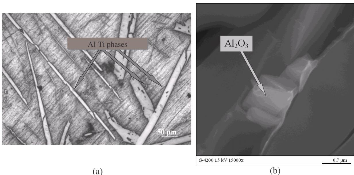
Fig.4. (a) Multicomponent phases in composites obtained *in situ* after synthesis Al-FeO·TiO<sub>2</sub> composite precursors at 1000 °C/1h, (b) Al<sub>2</sub>O<sub>3</sub> particle in composites.
