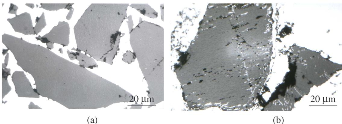
Fig.1: Structure of composite (a) after infiltration of loose ilmenite powder by liquid aluminium under 15 MPa pressure at  $640^\circ\text{C}$  (composite A), (b) after producing of suspension at  $700^\circ\text{C}$  (composite B).
