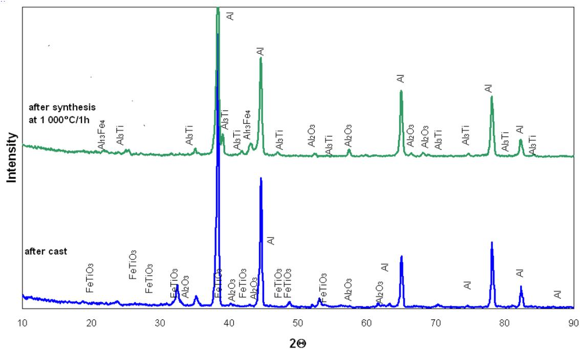
Fig.2. X-ray diagram of Al-FeO·TiO<sub>2</sub> system after producing of suspension at 700°C and after synthesise at 1000 °C.
