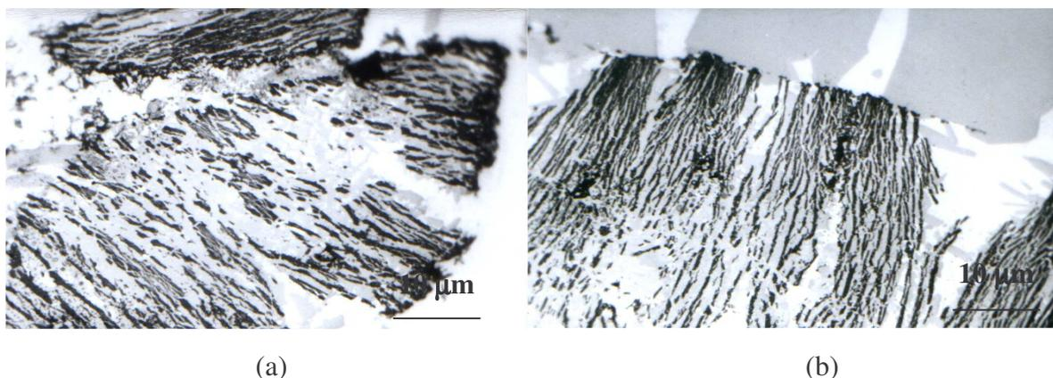
Fig 3. Structure of composite: (a) after synthesis of composite precursor A at 840 °C/1h, (b) after synthesis of composite precursor B at 1000°C/1h
