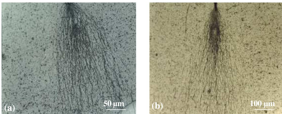
Figure 2. Optical micrographs of 4-point bending test at different magnifications
