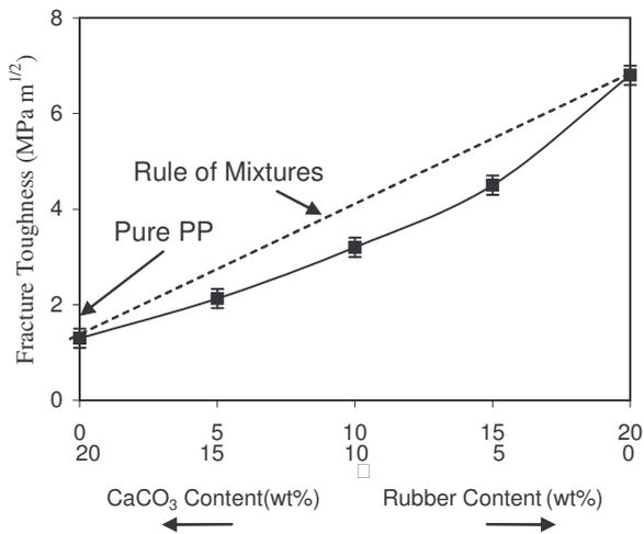
Figure 1. Variations of KIC of PP hybrid composite versus CaCO<sub>3</sub>/EPR ratio
