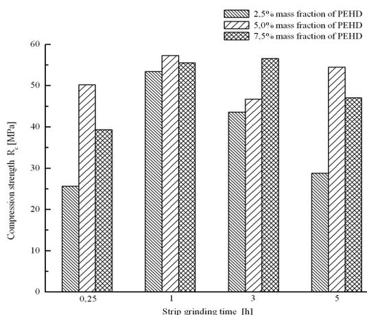
Fig. 4. Comparison of compression strength values of the investigated composites versus the PEHD mass fraction and strip grinding time
