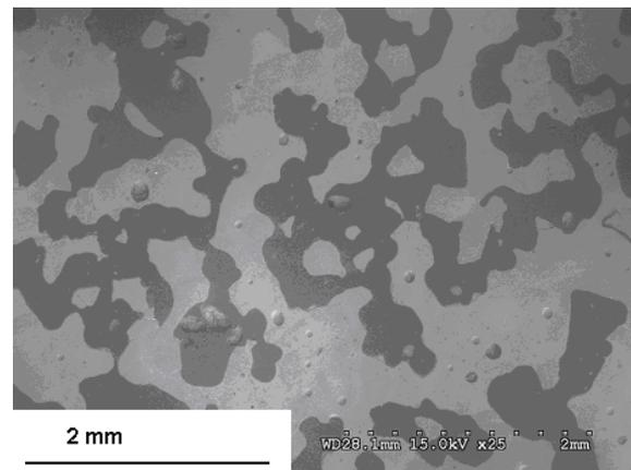
Figure 4. SEM image of surface of the ceramic-elastomer composites (S/G=1,50)
