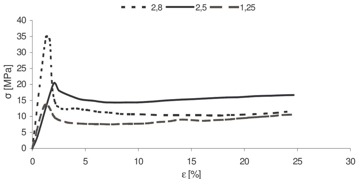
Figure 5. Diagrams of compression of composites infiltrated by elastomer with different hard segment content (S/G)
