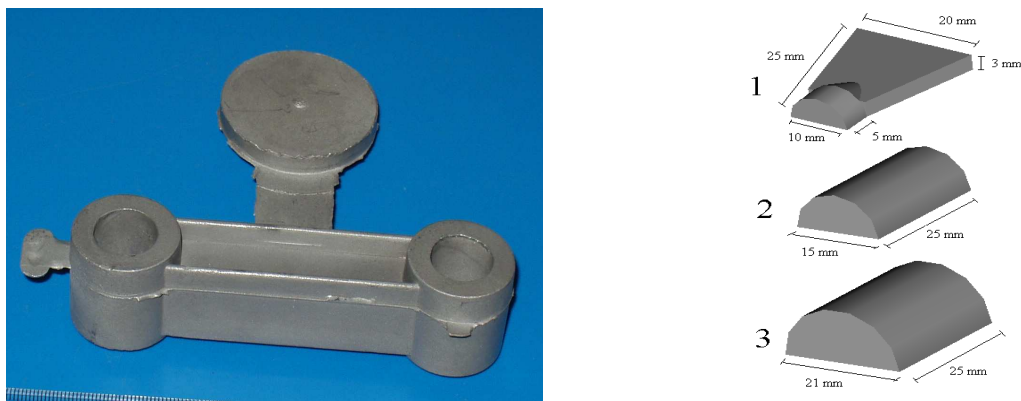
Figure 1. Typical thixocast part and schematic of the three gates employed in the experiments
