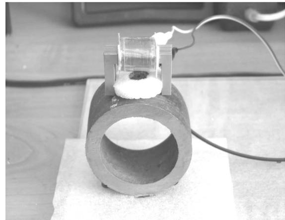
Figure 1. Schematic diagram of Barkhausen equipment Figure 2. Experimental set-up
