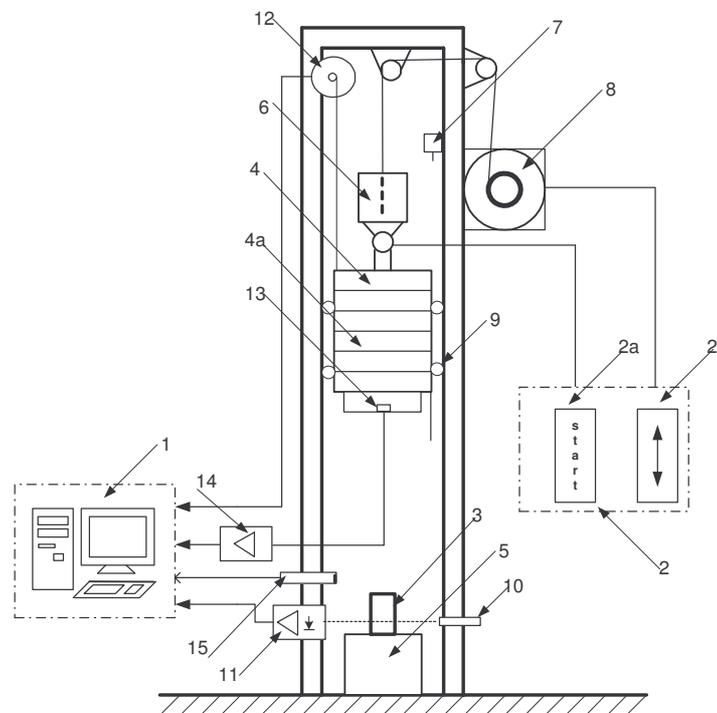
Figure 1. Investigation stan scheme: 1–data acquisition system, 2–hand control of ram displacement, 2a–ram release, 2b–ram position setting, 3–sample, 4–ram, 4a–hammer bobs, 5–anvil, 6–electromagnet, 7–limit switch, 8–electric motor, 9–rolling bearing, 10–laser transmitter, 11–exalted receiver, 12–rate generator piezoelectric sensor, 14–piezoelectric sensor amplifier, 15–distance sensor release
