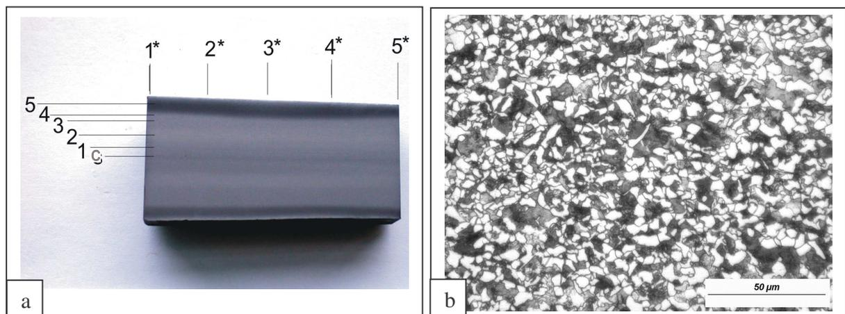
Fig.1. Specimen 3: (a) macrostructure in the longitudinal section, (b) LM micrograph of fine grain microstructure in the central part of specimen
