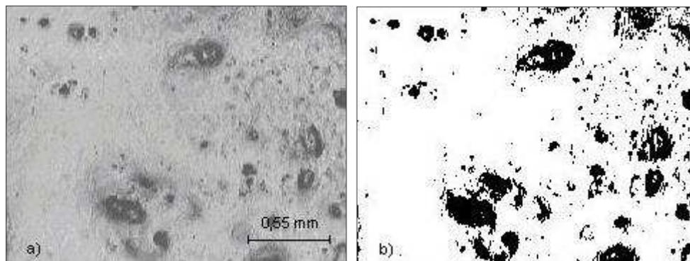
Figure 1. Monochromatic picture of deformed surface – a) and the same picture after binarisation with threshold 150 – b)
