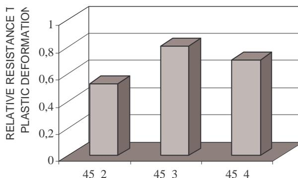
Figure 3. Relative resistance to plastic deformation measured for time T=20 min
