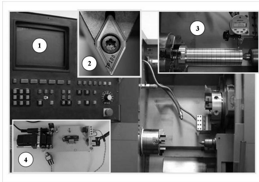
Figure 1. Experimental devices for the turning test and measurements of roundness: 1. CNC horizontal lathe equipped with a numerical control. 2. Tools used. 3. Digital-clock comparator. 4. Adapter to the RS-232 of PC.
