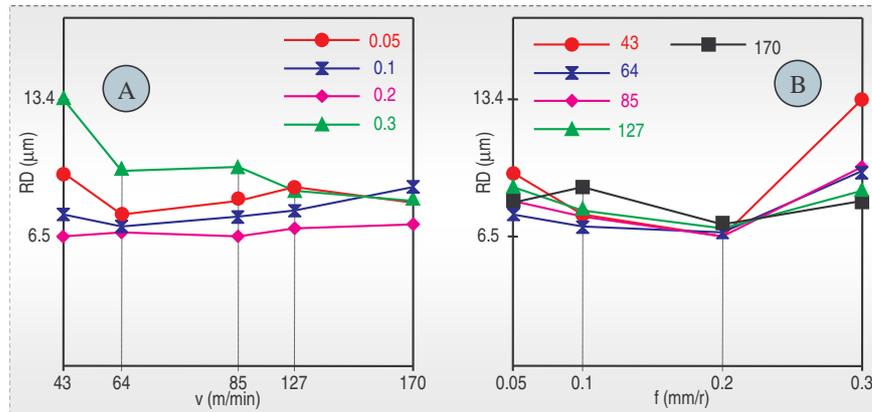
Figure 2. (a) Evolution de RD with  $v$  for  $f$  established. (b) Evolution of RD with  $f$  for  $v$  established
