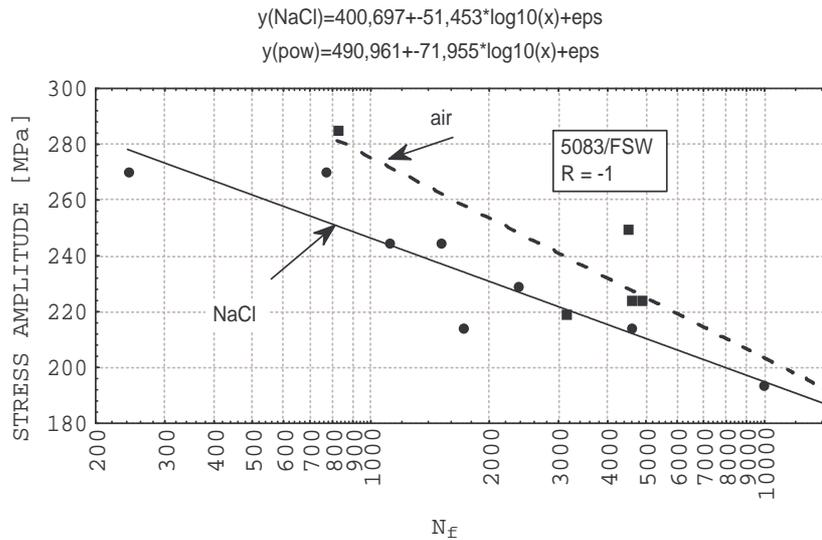
Figure 3. Low-cycle fatigue life for AlMg4,5Mn [5083] welded by FSW
