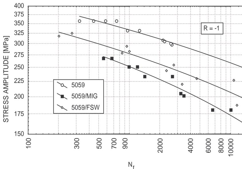
Figure 4. Low-cycle fatigue life of Alustar alloy, 5059 alloy welded by MIG and by FSW
