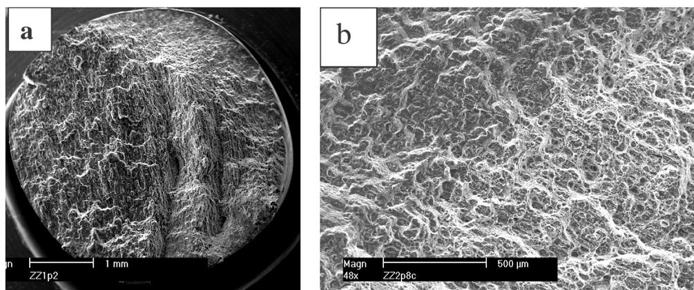
Figure 5. a) Fatigue fractures. The 5083 alloy welded by FSW method, tested in the air.
