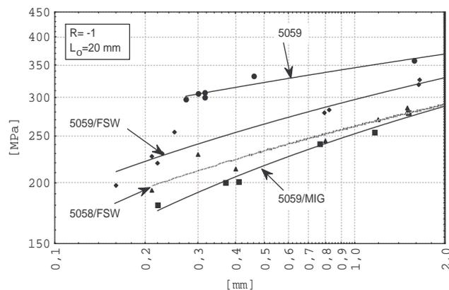
Figure 2. Diagrams of cyclic strain for the following: Alustar alloy (5059), Alustar alloy welded by FSW method (5059/FSW) and welded by MIG (5059/MIG) and AlMg4,5Mn welded by FSW (5083/FSW)
