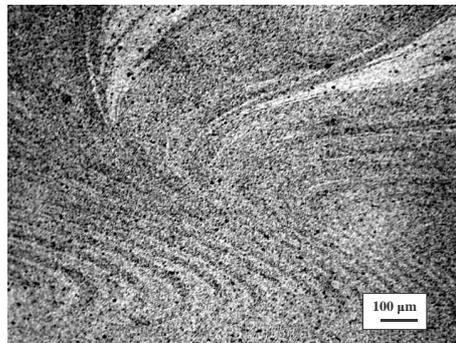
Figure 1. Microstructure of the weld's nugget of 5083 alloy
