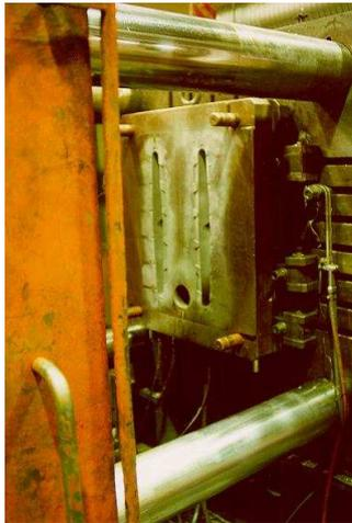
Figure 1. Fixed half of the die-casting die
