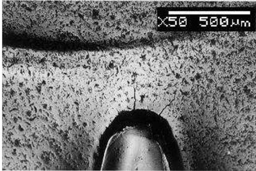
Figure 4. Working surface of the testing die-casting die. Surface crack and pits.
