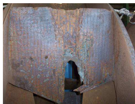
Figure 1. a) - a view of the fan of steel mill fumes suction system. Fan blades are covered by the wear plates 4666 CDP attached to the fan body by arc spot welding, b) - a view of worn center part of the fan blade
