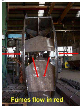
Figure 1. a) - a view of the fan of steel mill fumes suction system. Fan blades are covered by the wear plates 4666 CDP attached to the fan body by arc spot welding, b) - a view of worn center part of the fan blade
