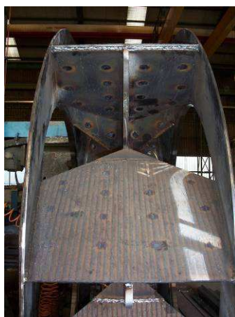
Figure 1. a) - a view of the fan of steel mill fumes suction system. Fan blades are covered by the wear plates 4666 CDP attached to the fan body by arc spot welding, b) - a view of worn center part of the fan blade
