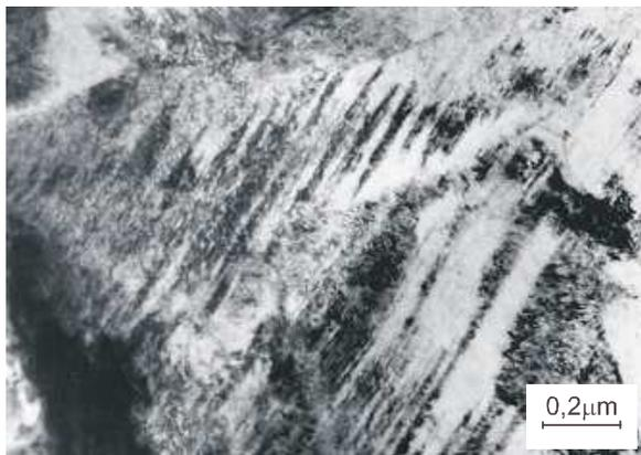
Figure 6. Structure of the lower bainite in TRIP-type sheets
