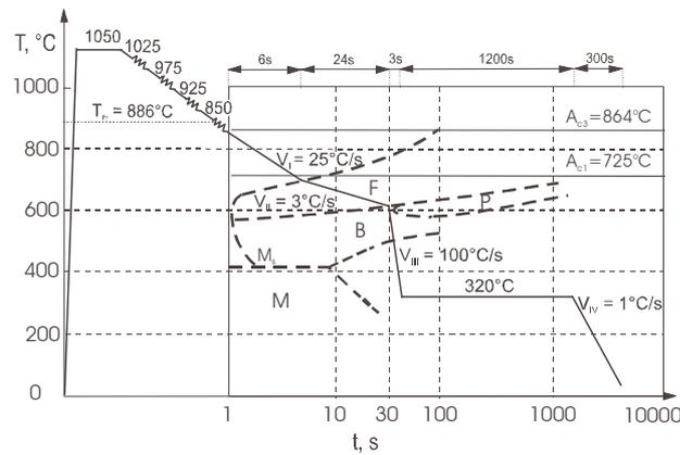
Figure 2. DTTT<sub>c</sub>-diagram of the investigated steel with marked cooling conditions of TRIP-type thermomechanically processed sheets
