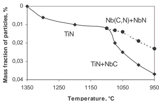
Figure 1. The temperature sequence of precipitation of MX-type phases in the austenite
