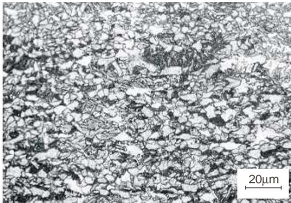
Figure 4. Fine-grained ferritic-martensitic structure of the thermomechanically processed sheet
