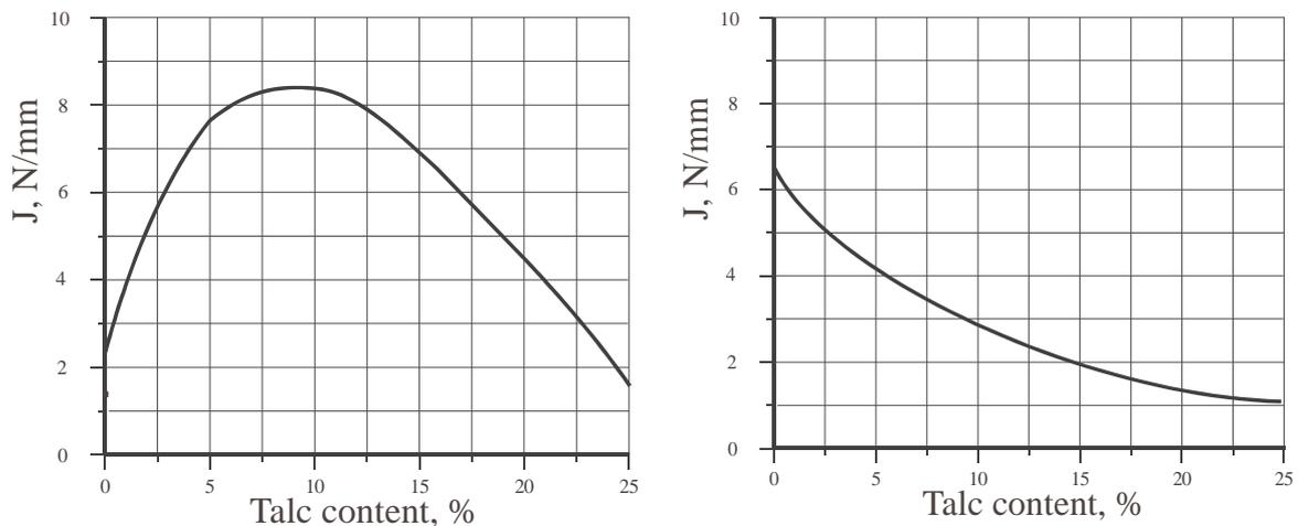
Figure 1. Influence of the filler (in form of talc) concentration on the value of integral J for different polymers a - PP; b – PA.
