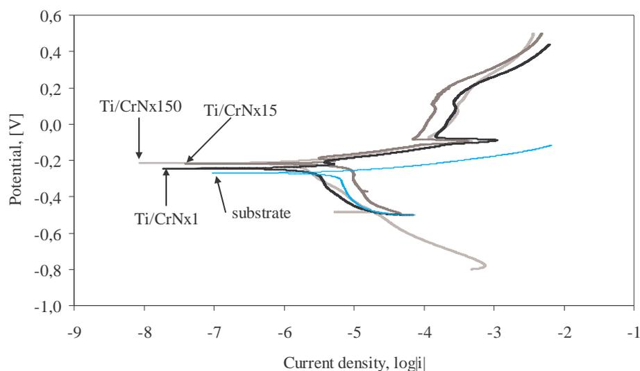
Figure 1. Potentiodynamic polarization curves of the Ti/CrN samples in 1 M HCl solution.
