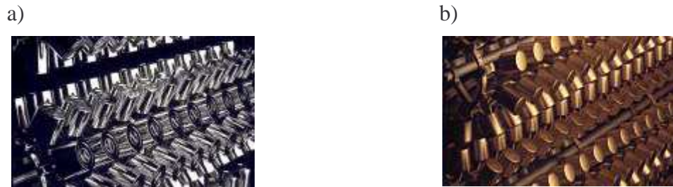
Figure 2. Products on plating racks painted with a) colorless lacquer, b) dye lacquer (gold)
