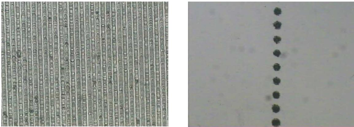
Figure 1. Optical micrographs of: a) texture structure, b) single groove (700 mm/s, 2 kHz)
