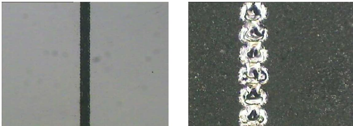
Figure 2. Optical micrographs of grooves for: a) 100 mm/s, 40 kHz, b) 600 mm/s, 5 kHz,
