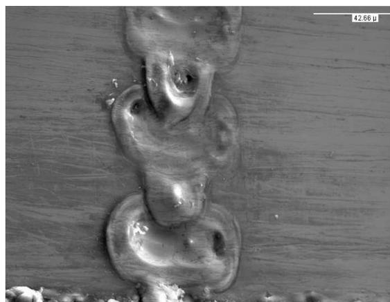
Figure 3. SEM micrograph of groove: 600 mm/s, 5 kHz
