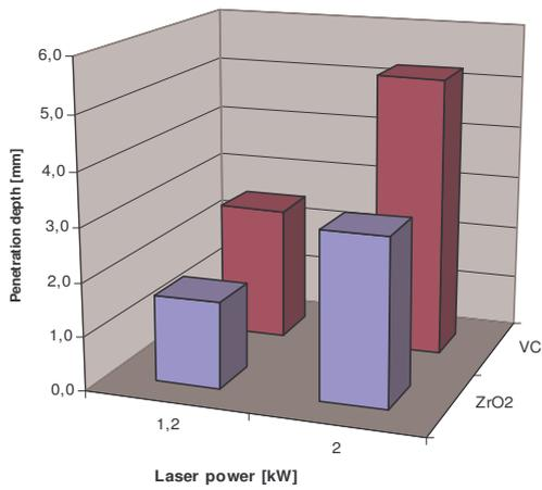
Figure 4. Plot showing the remelting laser power effect on the remelting zone depth
