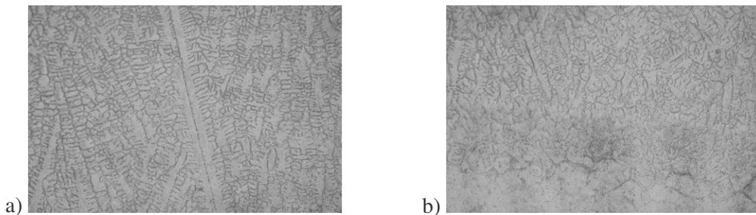
Figure 2. Surface layer structure of the test piece from the X40CrMoV5-1 tool steel after alloying with the  $\text{ZrO}_2$  ceramic powder using the HPDL diode laser, a) magnification 100x, b) magnification 200
