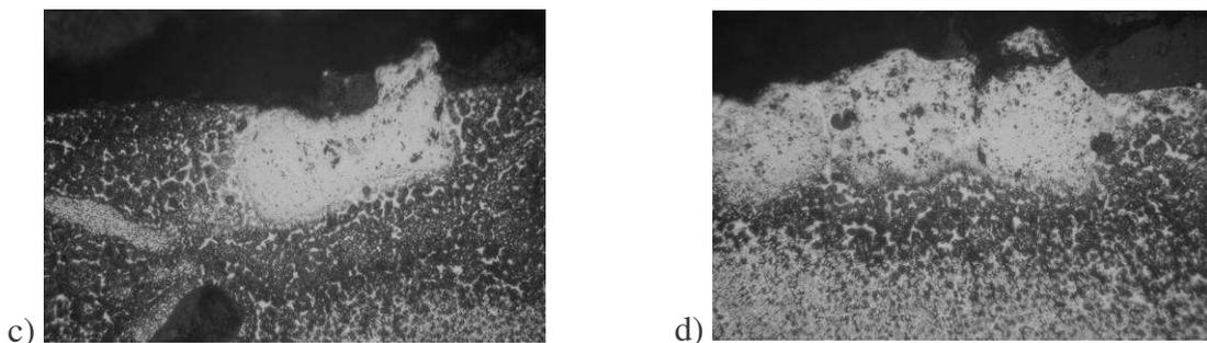
Figure 3. Surface layer structure of the test piece from the X40CrMoV5-1 tool steel after alloying with the VC ceramic powder using the HPDL diode laser, c,d) magnification 100x
