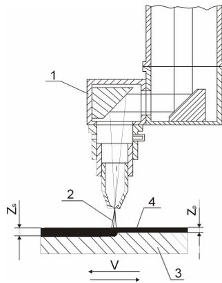
Figure 1. Schematic diagram of the laser alloying process, due to remelting the substrate material with the alloying material layer put down on it: 1 – laser focusing system, 2 – laser beam, 3 – alloyed material, 4 – alloying material,  $Z_s$  - depth of the alloyed layer,  $Z_p$  - thickness of the alloying layer.
