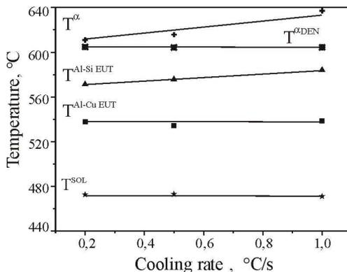
Figure 2. Influence of the cooling rate on the temperature:  $T^\alpha$ ,  $T^{\alpha DEN}$ ,  $T^{Al-Si EUT}$ ,  $T^{Al-Cu EUT}$ ,  $T^{SOL}$
