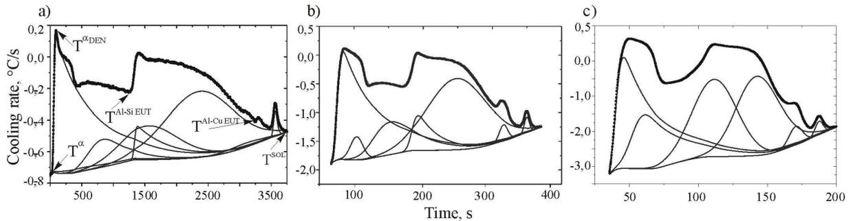
Figure 1. Derivate curves with peak fitting for cooling rate: a) 0,2 °C/s, b) 0,5 °C/s, c) 1 °C/s
